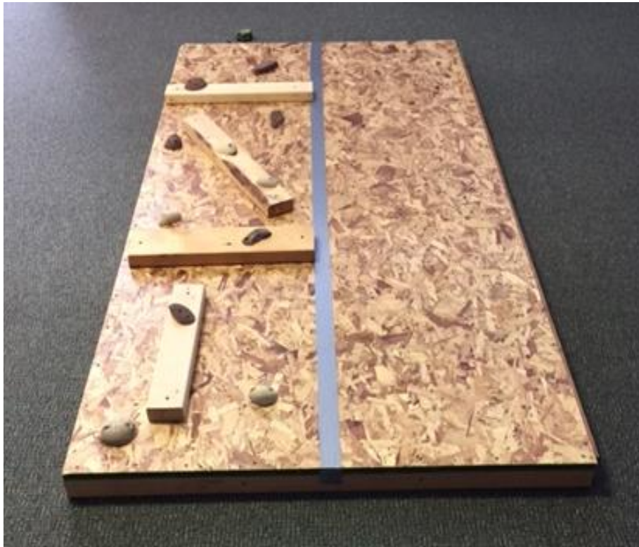
Figure 1: Photo of the running section. Left represents the uneven terrain right the even terrain.
