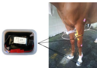
Figure 1: The sensor unit in the casing (left) and the four sensors mounted on forearm and hoof (right).
