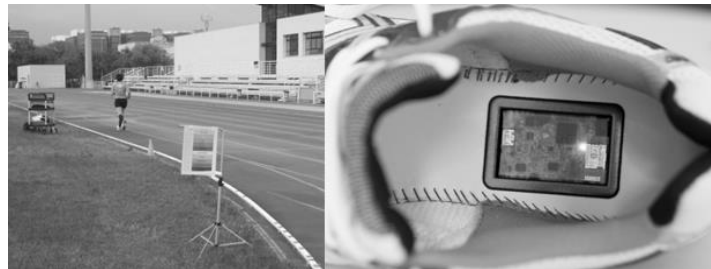
Figure 1: Runner during a constant-speed test (left) and IMU integrated in the midsole (right).
