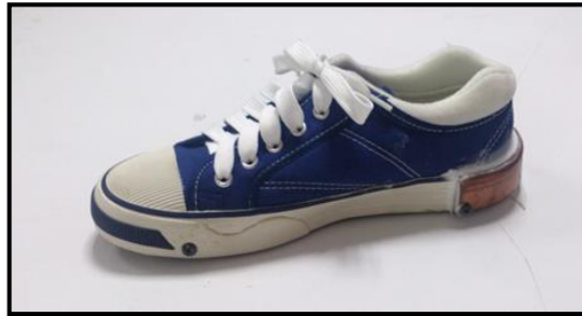
Figure 1: Shoe E of which with a curved metal block of 200 grams screwed in the rear end.
