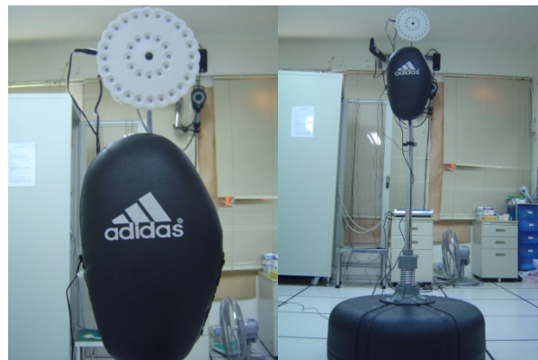
Figure 2: The instrumented kicking target and the starting signal for the karate athlete.
