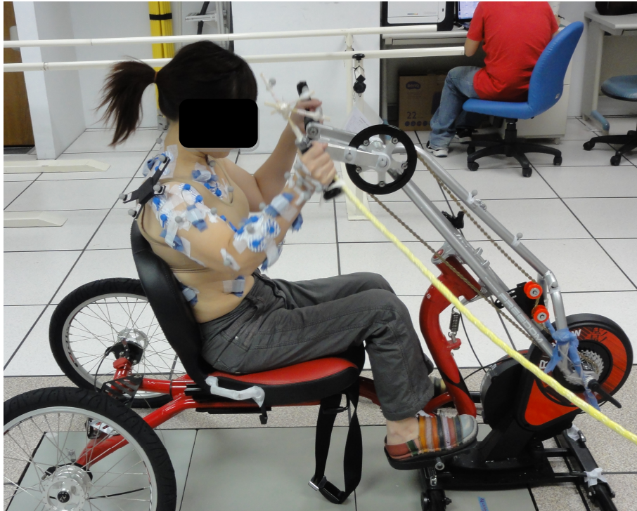
Figure 1: A subject performing handcycling on a handcycle with its front wheel replaced by a resistance training platform. The handgrip was instrumented with a 6-component load cell to measure the handgrip reaction forces. The seat could be moved horizontally and vertically to the tested positions.
