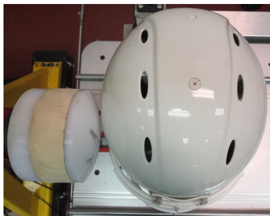
Figure 1: The front boss positive azimuth location shown on a typical American football helmet. A striker cap is shown to demonstrate the possible complex interactions between the helmet shell and liner for this type of non-centric location.
