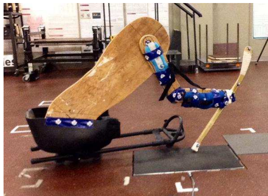
Figure 1: Illustration of the validated solid-static prototype used to determine baseline measures for the preparation phase within the sport of sledge hockey (not test position).
