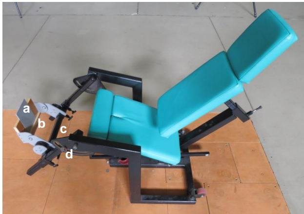
Figure 1. Purpose-built chair for chair measurements, a = foot platform, b = shelf to support heel and preventing slipping off platform, c = steel frame for adjustment leg size, d = leg frame for adjustment knee angle.
