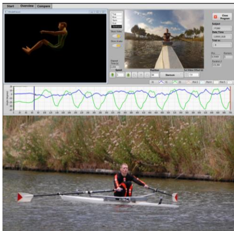
Figure 1: Details of the setup and recording and analysis software. Recording tablet and wireless dongle are mounted in a box on deck behind the rower. Camera's on both decks.
